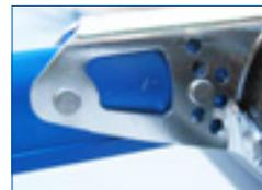
Insert the wire into the larger of the two slots in the fitting at the outboard end of the spreader and tighten the screw to hold it securely. The spreader length should be set at 19" from the side of the rig to where the wire intersects the spreader.
