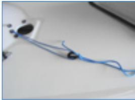
line up through the inboard bullseye on the starboard side of the deck at the mast partners, through a single 29mm with stainless steel strap, and tie it off to the eye strap at the mast step.
