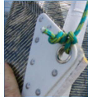
Feed the sail into the track and hoist until the inner end of the first batten pocket is in the track. Insert the upper batten into the top pocket with the soft end in first. Put moderate pressure on the batten and secure the outboard end. Raise the sail to the second batten pocket and install the second batten.
