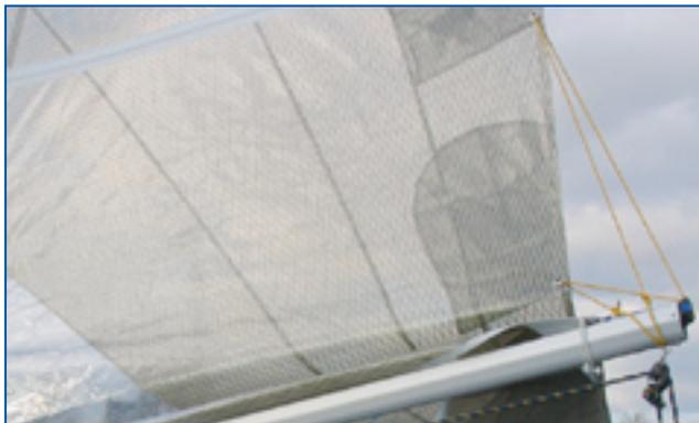
of the excess line out of the forward part of the boom, making sure it is led through the fairlead on top of the boom at the gooseneck.
