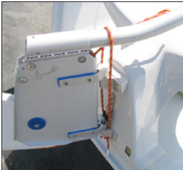
Pass the tiller under the traveler and into the rudder head, and insert the cotter pin into the top of the tiller at the aft end to lock it in place. Install the tiller extension onto the tiller, making sure the fitting snaps into place securely.
