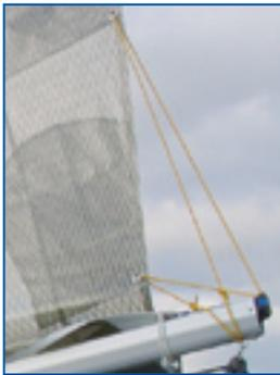
**Reef Lines** Hoist to the second reef point and rig the second reef line, which is the one on the port side of the boom. Hook the reef line in to the grommet in the luff of the sail; then run the aft end of the line through the grommet in the leech. Tie a tight bowline around the boom through the eye strap holding the aft mainsheet block.
